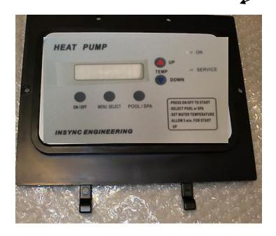
FIGURE 4 - PASTE ON NEW INSYNC KEYPAD, ALIGNING CONNECTOR THROUGH OPENING, AND MAKING SURE FEATURES IN THE PLASTIC ALSO LINE UP. IF YOU MAKE A MISTAKE, HEAT UP THE PANEL AND MOVE IT AROUND.
