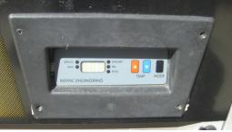
STEP 1. ALL OF THESE HAYWARD PANELS ARE THE SAME FIRST REMOVE THE PLASTIC PANEL. YOU MAY HAVE TO GET TO THE SCREWS FROM THE FRONT (AS SHOWN) OR ON SOME FROM THE BACK
