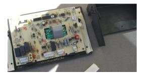
STEP 4. YOU SHOULD NOW BE ABLE TO SEE THE KEYPAD CONNECTION. UNPLUG IT AND THEN IF YOU CAN REMOVE THE OLD KEYPAD FROM THE FRONT PLASTIC. YOU MAY HAVE TO LOOSEN THE SCREWS ON THE PRINTED CIRCUIT BOARD TO REMOVE THE CONNECTOR TAIL.
