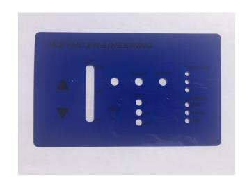
NEW ADHESIVE IS "PRESSURE SENSITIVE" SO USING KLEENIX OR SOFT CLOTH, RUB FRONT OF LABEL WHERE IT ATTACHES TO METAL APPLYING PRESSURE TO ACTIVATE ADHESIVE
