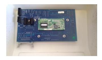
TRY NOT TO TOUCH ANY OF THE CIRCUIT CARDS TO AVOID DAMAGING THEM. REMOVE 4 SCREWS SECURING BOARD TO HOUSING
