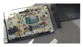
STEP 4. YOU SHOULD NOW BE ABLE TO SEE THE KEYPAD CONNECTION. UNPLUG IT AND THEN IF YOU CAN REMOVE THE OLD KEYPAD FROM THE FRONT PLASTIC. YOU MAY HAVE TO LOOSEN THE SCREWS ON THE PRINTED CIRCUIT BOARD TO REMOVE THE CONNECTOR TAIL.
