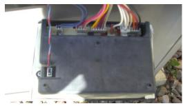
STEP 2. REMOVE ALL THE CONNECTIONS AT THE BACK. THE CONNECTORS ARE ALL KEYED BUT YOU MAY NEED TO TAKE A PICTURE TO REMEMBER HOW TO HOOK IT BACK UP
