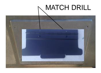
PLACE COVER APPROXIMATELY WHERE SHOWN AND MATCH DRILL 2 ATTACHMENT HOLES INTO YOUR EXISTING PLASTIC. USE .060 TO .070 DIA DRILL BIT. SCREW HINGE TO PLASTIC BEZEL USING SELF TAPPING SCREWS
