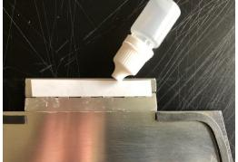
APPLY ADHESIVE TO BACKSIDE OF INDICATED "FIXED" SECTION ON COVER HINGE. DO NOT GET ADHESIVE ON "SWINGING" SECTION OF COVER HINGE
