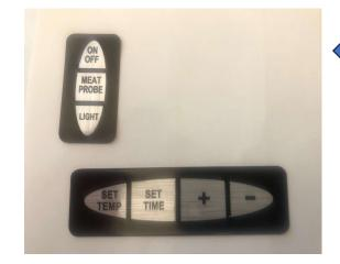
REMOVE YOUR NEW OVERLAYS AND POSITION CAREFULLY OVER THE EXPOSED BUTTON OPENINGS, ALIGNMENT IS RIGHT IN THE CENTERLINES VERTICAL AND HORIZONTAL OVER THE BUTTON OPENINGS
