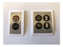
REMOVE YOUR NEW OVERLAYS AND POSITION CAREFULLY OVER THE EXPOSED BUTTON OPENINGS, ALIGNMENT IS RIGHT IN THE CENTERLINES VERTICAL AND HORIZONTAL OVER THE BUTTON OPENINGS
