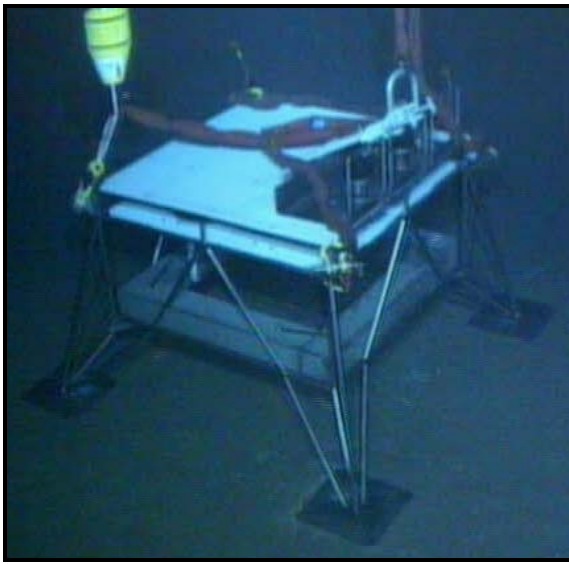
Figure 14. Anode deployed on the seafloor at a depth of 2380 meters offshore Cyprus
