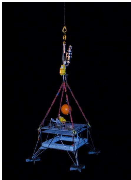
Figure 12. Anode assembly during deployment
