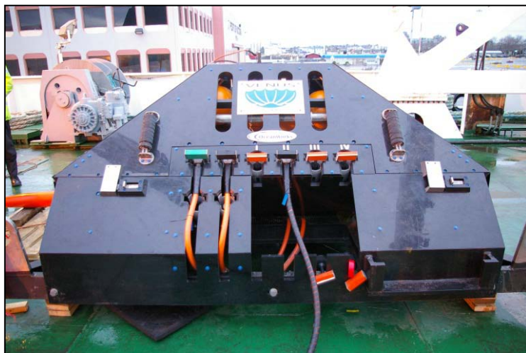
Figure 5. Node base with retrievable node installed, input power, input optical signal connected and 1 of 4 instrument connected.
