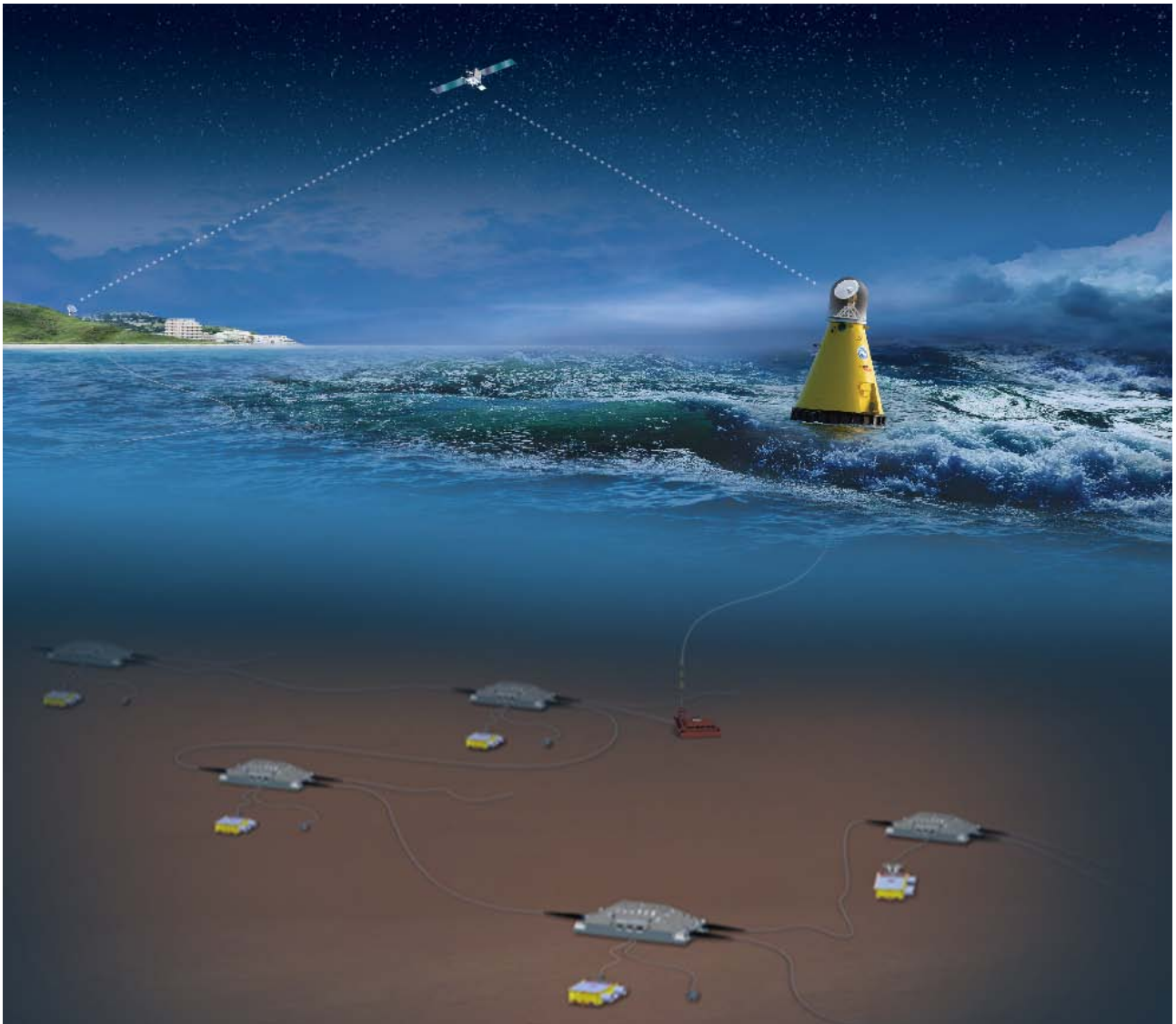
Figure 3. Science observatory network architecture with backbone cable, nodes, sensors, and electrical power.
