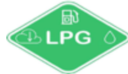
Fig 2. Vehicle powered by LPG in J3108-1 and ISO 17840 formats. Common lettering is maintained but the J3108-1 format retains the existing NHTSA Safety Blue color to prevent responders associating the green more commonly used in North America to depict oxygen, inert gasses, and safety.
