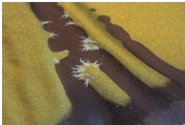
Figure 1 Photo of Dendrites in Windings of Cell 5 (100% SOC) from Battery 412 (gold color shows a high charged region and the brown shows a lower charged region)
