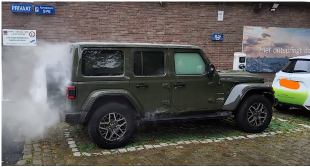
Fig 2. Jeep plug-in hybrid undergoing battery failure was hard to differentiate from non-hybrid Wranglers. The cabin was full of flammable vapors. (Belgium 10/30/23)
