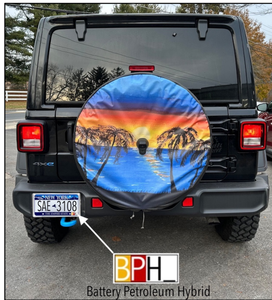
Fig. 4. SAE J3108 license plate marking (sticker) for firefighter awareness about alternative fuels and power sources.
