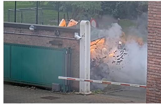
Fig. 3. Jeep exploded after firefighters broke a window to ventilate the interior. Note firefighters in blast.
