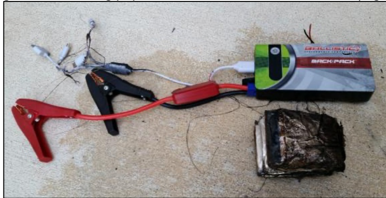
Fig. 9. Damaged consumer items emit flammable and toxic fumes, as shown with this new versus burnt booster pack.
