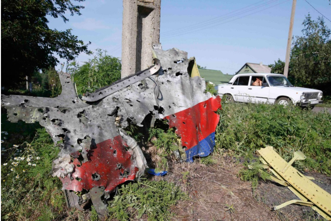
Figure 2. Shotgun type of damage inflicted on structure on a Boeing 777, operating as MH17 when shot down over Ukraine in July 2014. (Press)
