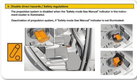
The Volvo XC60 PHEV emergency response guide shows how to disconnect the high-voltage battery by locating a plug in the floor between the rear seats.
