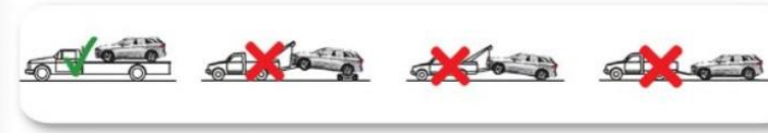
The Volvo Emergency Response Guide is typical in only permitting use of a flatbed/rollback to move vehicles. Source: Volvo Emergency Response Guide
