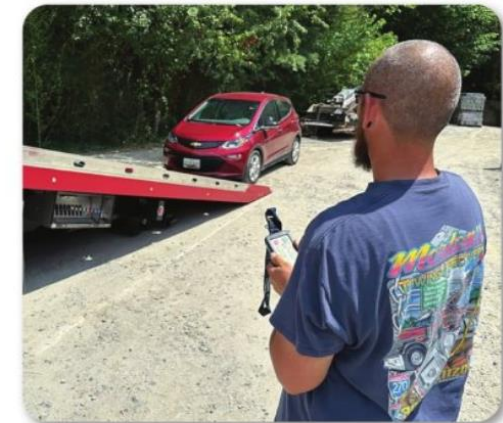
Brian Jones of Morton's Towing and Recovery demonstrates use of a wireless remote to load an EV. The car is downwind from where he is standing. It can be dangerous to use the controls located beneath the bed.
