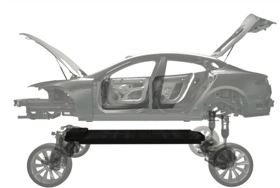
Figure 1. The body (gray) and battery (black) of the Tesla Model S are separate structures. Water in the body will drain out the doors without cooling the battery. Between these separate structures are typically layers of acoustic insulation and waterproofing which can further shed water. 2
