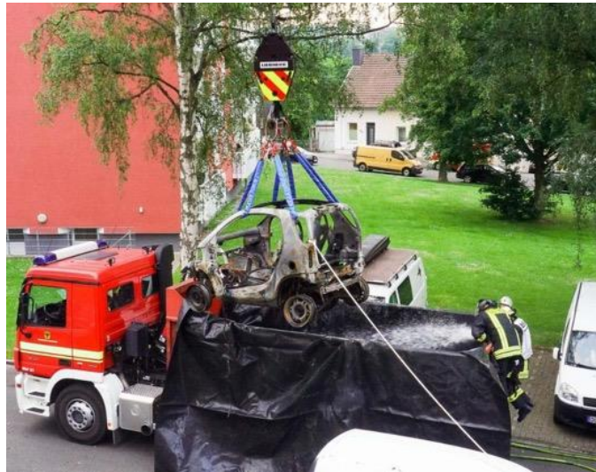
Figure 9. Ad hoc equipment for immersion of electric auto. 10
