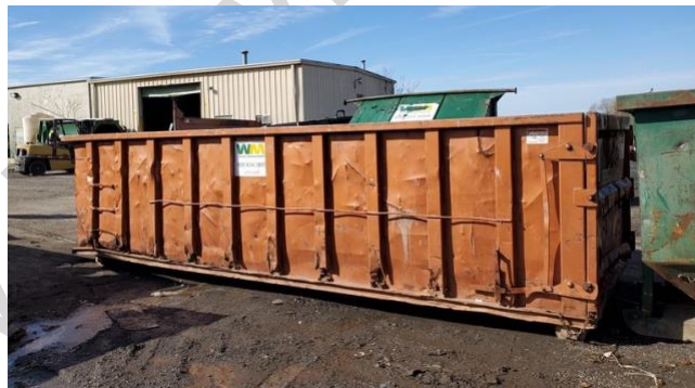
Figure 10. Photo of an open top roll off dumpster with a side hinged rear door.
