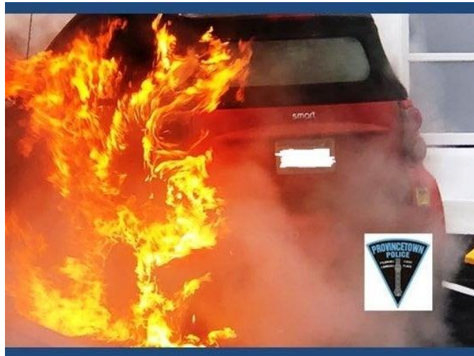
Figure 3. This burning electric vehicle is too close to the ground to cool the bottom of the battery and venting flame along the rocker panel prevents jacking from at least the near side to expose the bottom of the battery. 4
