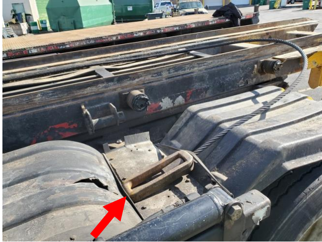
Figure 11. The end of the roll-off truck cable which is used to deliver the container could be also be used to drag a vehicle into the dumpster.
