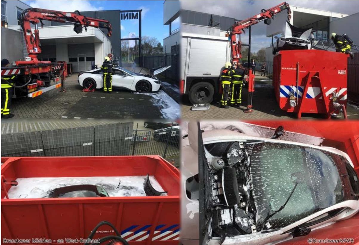
Figure 8. Smoking BMW i8 placed in water for 24 hours. 9
