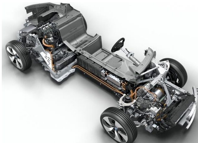
Figure 5. The BMW i8 battery is in a central tunnel minimizing exposure to cooling the bottom of the vehicle.
