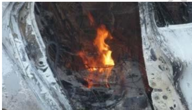
Figure 6. Renault Zoe battery fire during test. Rear seat cushions have been removed. 7
