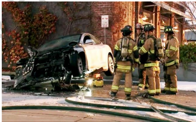
Figure 2. Tesla Model S extinguished by lifting side of car to cool the bottom of the battery. This car re-ignited twice more over a 16 hour period. 3
