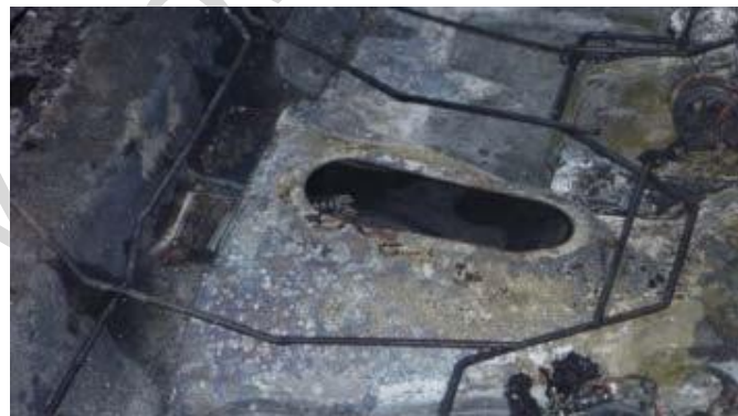
Figure 7. Opening beneath rear seat following Renault Zoe battery fire test. 8
