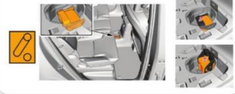
The Volvo XC60 PHEV emergency response guide shows how to disconnect the high-voltage battery by locating a plug in the floor between the rear seats.
