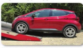
Stopping at this point allows the tow operator to examine the bottom of the battery for road damage and hot areas. Check the rear wheels so the EV cannot inadvertently roll backward.
