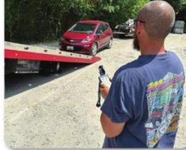
Brian Jones of Morton's Towing and Recovery demonstrates use of a wireless remote to load an EV. The car is downwind from where he is standing. It can be dangerous to use the controls located beneath the bed.
