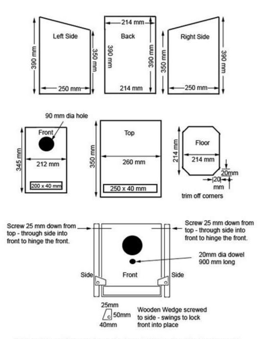
Preferred timber 18mm exterior grade plywood. The box is not glued but screwed together with galvanised screws. Also the box is not painted so not harmful fumes. Trim the coners off the floor as shown to allow for drainage. The front is hinged and held in place with two wooden catches, this has proved to be a very good all purpose box, not only for possums but gliders seem to like it and birds also! By having the front hinged it allows easy access to animals in care and for cleaning.
