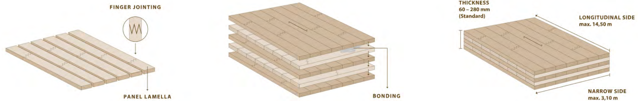
128mm CLT Cross Laminated Timber
