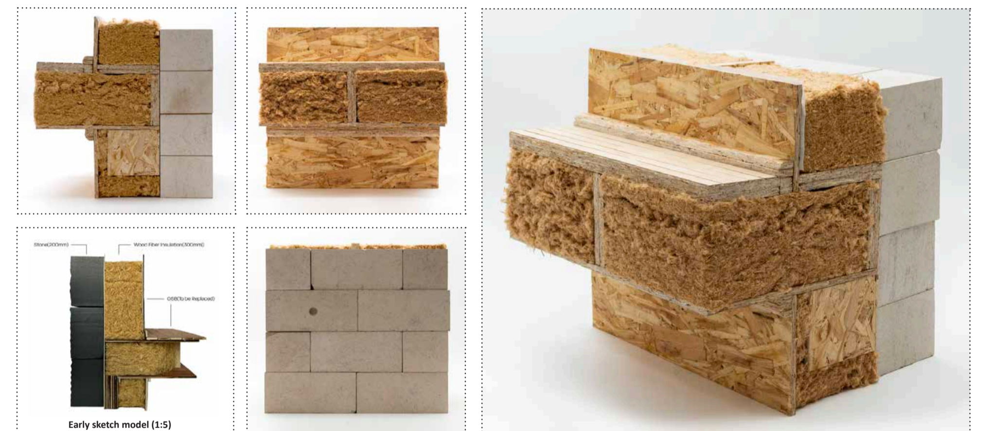
1:2 SCALE MODELS OF THE ATTEMPTED "NET-ZERO" NATURAL FIBRE (ABOVE) AND GLASS FIBRE (BELOW) INSULATED STONE-OSB WALL BUILD-UP
