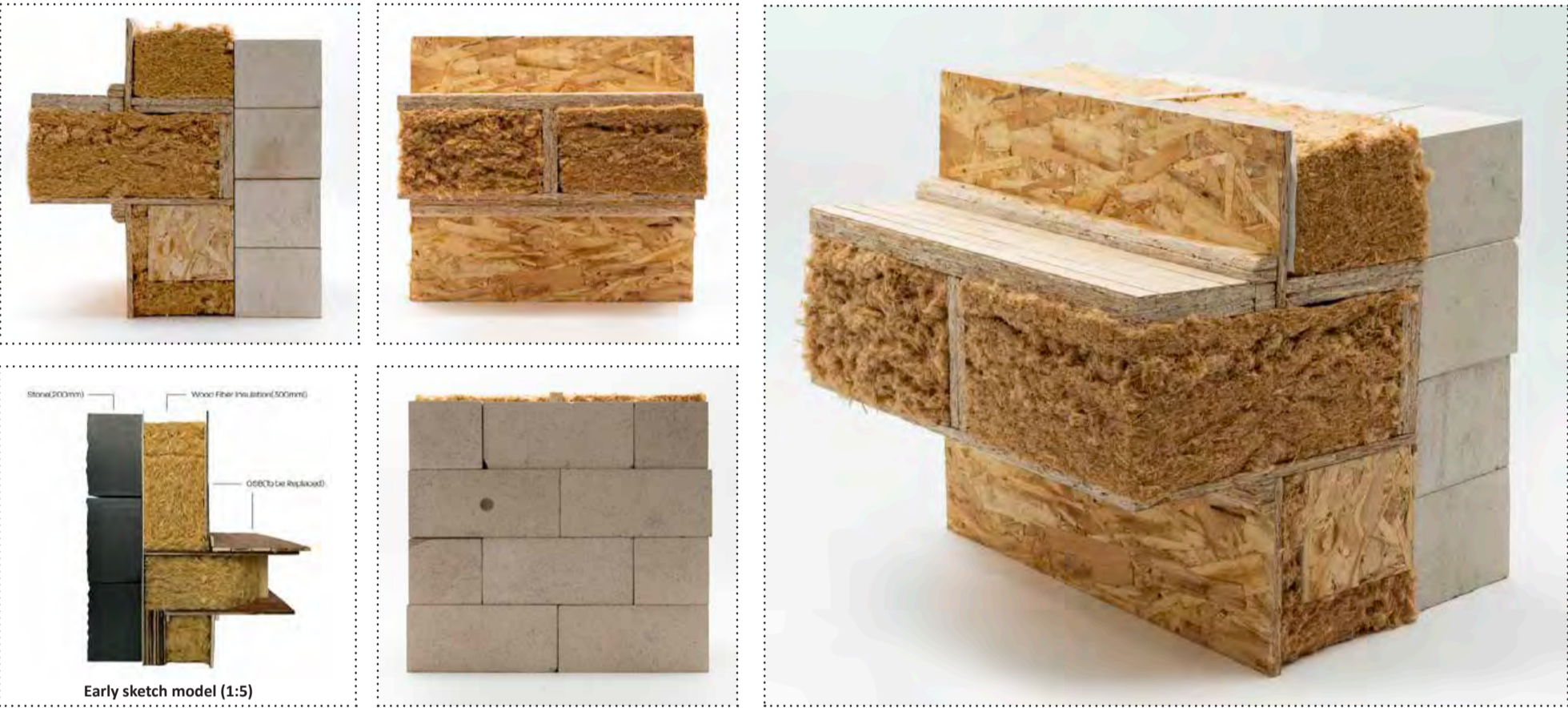
1:2 SCALE MODELS OF THE ATTEMPTED "NET-ZERO" NATURAL FIBRE (ABOVE) AND GLASS FIBRE (BELOW) INSULATED STONE-OSB WALL BUILD-UP
