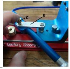
5. Back OD cutter (a) off all the way on the cutter body by turning cutter depth adjustment knob (b) counter clockwise. This will allow clearance to place cutting arbor in place and for initial trimming set-up.
