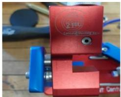
7. Cutter body should be at an angle where you can see the trimming operation. Roughly a 45 degree angle or more.
