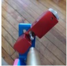
8. Place the cutting arbor into the cutting body so the cutter and slot in arbor are facing outward. Shown on image (a.) Flat on shank of arbor should be facing the dial side. The cutter face on the arbor should just be slightly to the right of a line perpendicular to the left side of the outside cutter (blue line image b.). Tighten arbor into place with arbor tensioning bolt with a 5/32" allen wrench. Keep a good space between outside cutter and arbor to allow neck clearance when setting up.
