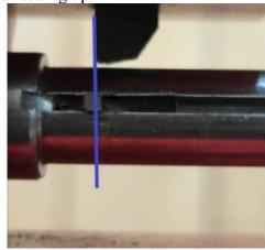
9. Take the O-Ring off the end of the driver on the case holder driver. This eliminates any variances the flexibility the o-ring may cause.
