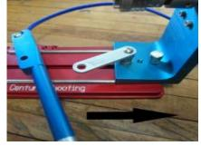
\*\*\*Push down on linkage arm while pulling pin. Also use extreme caution not to pull on the power handle cord!
