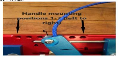
4. Place L-Bracket with power housing back onto base by depressing button (a) and carefully sliding bracket back into base slot. Swing handle linkage (b) to line up with pin hole on handle and Replace brass pin (c).
