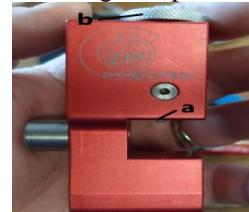
6. Attach cutting body to left L-bracket with tool body screw (A) with the two aluminum spacers (B) on screw on the inside of bracket as pictured. Tighten screw (A) with 5/32" Allen wrench so that the cutter body is tight against the L-Bracket and the spacers without any play. Note (Do not use the rubber flat washers that are used in the neck turning set-up) Do not over tighten.
