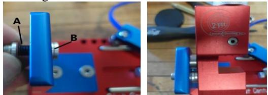
7. Cutter body should be at an angle where you can see the trimming operation. Roughly a 45 degree angle or more.
