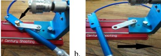
a. **\*\*\*Push down on linkage arm while pulling pin. Also use extreme caution not to pull on the power handle cord!**
