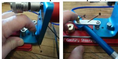
5. Back OD cutter (a) off all the way on the cutter body by turning cutter depth adjustment knob (b) counter clockwise. This will allow clearance to place cutting arbor in place and for initial trimming set-up.
