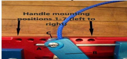
4. Place L-Bracket with power housing back onto base by depressing button (a) and carefully sliding bracket back into base slot. Swing handle linkage (b) to line up with pin hole on handle and Replace brass pin (c).
