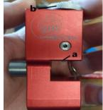
6. Attach cutting body to left L-bracket with tool body screw (A) with the two aluminum spacers (B) on screw on the inside of bracket as pictured. Tighten screw (A) with 5/32" Allen wrench so that the cutter body is tight against the L-Bracket and the spacers without any play. Note (Do not use the rubber flat washers that are used in the neck turning set-up) Do not over tighten.
