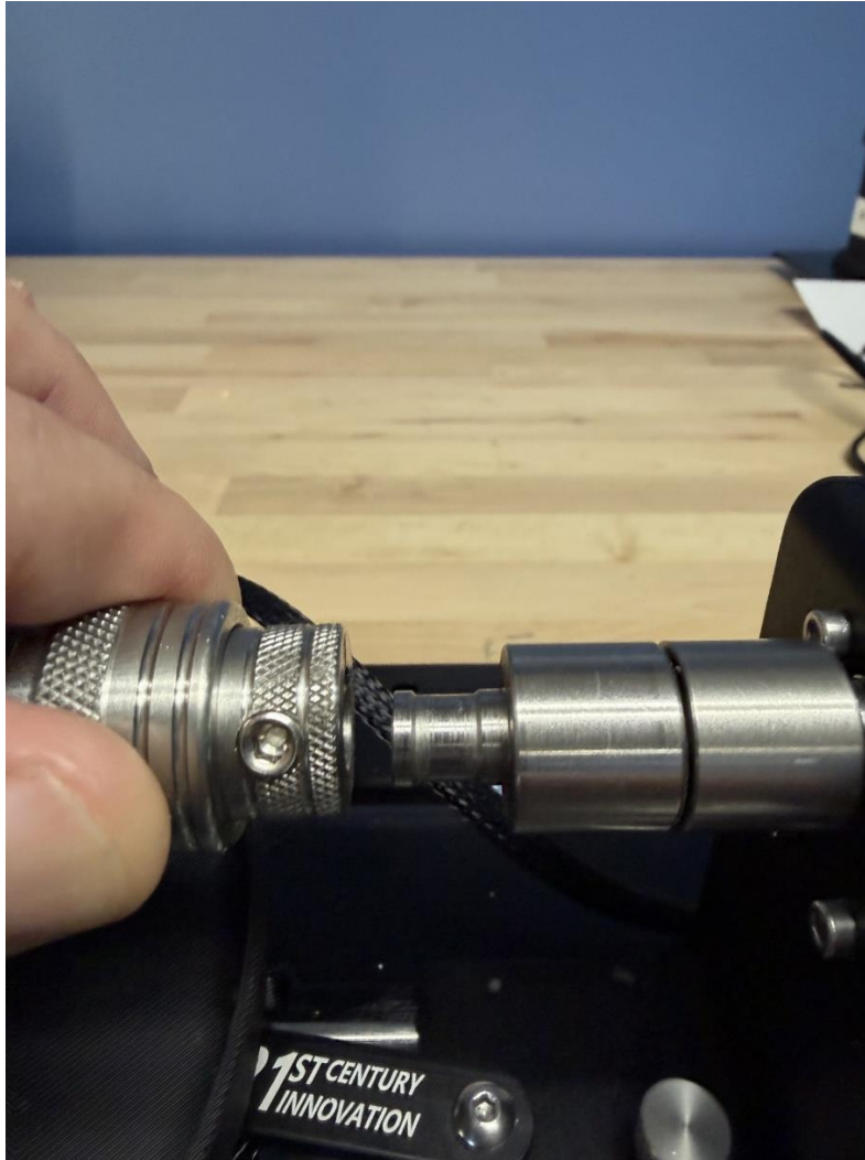
Installing the Case Holder and Driver on the Shaft Coupling.
