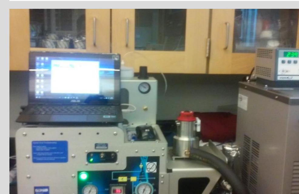
High Pressure Processing Unit (Barocycler Hub440, Pressure BioScience Inc., South Easton, MA) equipped with water jacket and circulating water bath for precise application of hydrostatic pressure at controlled temperature. Public Health Microbiology Laboratory, TSU.
