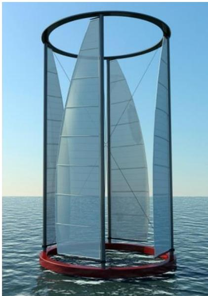
American Offshore Energy takes a page out of the Americas Cup sailboat design technology to build a high tech, low cost, floating, Vertical Axis Wind Turbine (VAWT). The aerodynamic section of this VAWT is built with a combination of tension and compression design principles allowing for stiff light weight structures that can scale to large size. The low center of gravity and broad support base makes for a stable floating wind turbine design.
