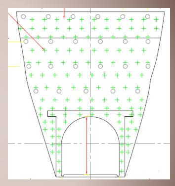
The slope stabilization of the entire area needs to be done to provide the vertical face for portal. Tunnel portal is excavated through vertical face and usually provided till the tunnel gets the cover of 2D, where D= Tunnel Diameter. Portal is usually been supported with steel ribs and shotcrete.
