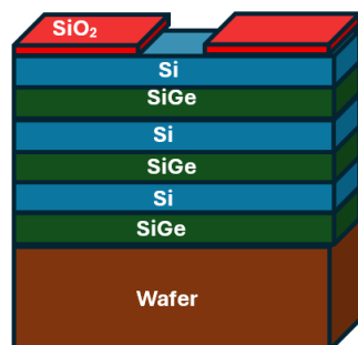
Fig 12(b) The pattern for each nanosheet segment is defined using SiO 2 protection layer. Unprotected regions will be etched away.
