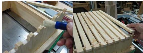
Glue the ends and attach the bars, nail.
