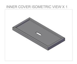
The inner cover as shown is probably the most difficult part to build. Having slots cut into the side rails to accept a ¼" piece of plywood. If this is too difficult, consider using off cut pieces to sandwich the plywood creating rails of similar dimensions.
