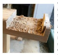
wood with a chisel. This can also be done using a circular saw. This took a lot of extra time but turned out well and the box assembled easily. On subsequent Nucs I used my router table to remove ¾" wide by 3/8" deep of material and that made short work of the end
