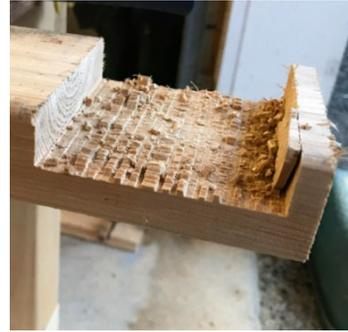
wood with a chisel. This can also be done using a circular saw. This took a lot of extra time but turned out well and the box assembled easily. On subsequent Nucs I used my router table to remove 3/4" wide by 3/8" deep of material and that made short work of the end
