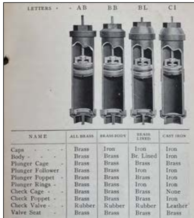
Top: Diagram of pumping cylinder (Baker, Field Guide, 19)
