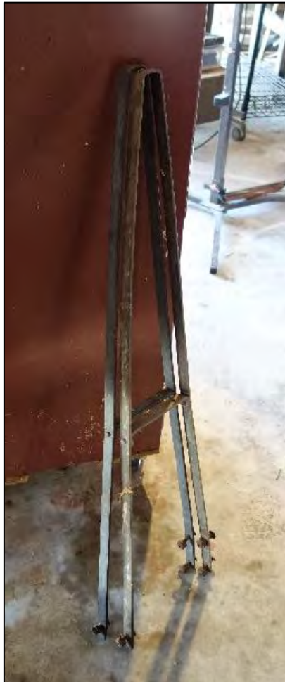
Above: Two arms of the wheel were salvaged from the Scandia barn. The arms match the wheel arm (Part 32—at the top of the diagram) in a pre-1898 Aermotor catalog. (“Early Bell Hub Parts,” http://www.vintagewindmillpartslist.com/id1.html )
