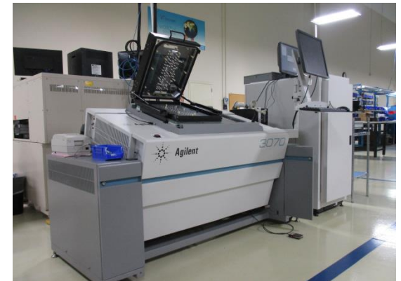
In – Circuit Test
