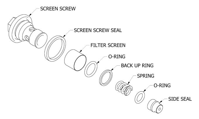
**CAUTION!** To avoid possible contamination by the residual chemical inside the Gun do not interchange the Isocyanate (A) parts with the Polyol (R) parts. The Isocyanate (A) side is identified with an (A) on the Screen Screw Head and the Polyol (R) side is marked with an (R) on the Screen Screw Head. The Gun Block is also marked with (A) and (R) designation.
