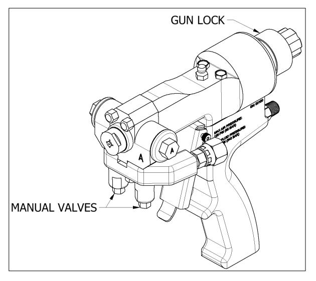
WARNING! Before proceeding with any maintenance work on the AP-3 Gun, trigger the gun to remove internal material pressure, ensure the Manual Valves are CLOSED, ensure the Gun Lock is in the LOCKED position, and SHUT OFF/DISCONNECT the air supply. It is recommended to remove the Gun from the Coupling Block.
