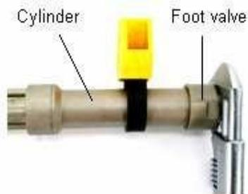
1. Remove the foot valve while holding the cylinder with a strap wrench.
