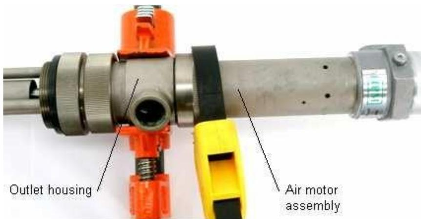
Use a strap wrench to remove the air motor assembly.
