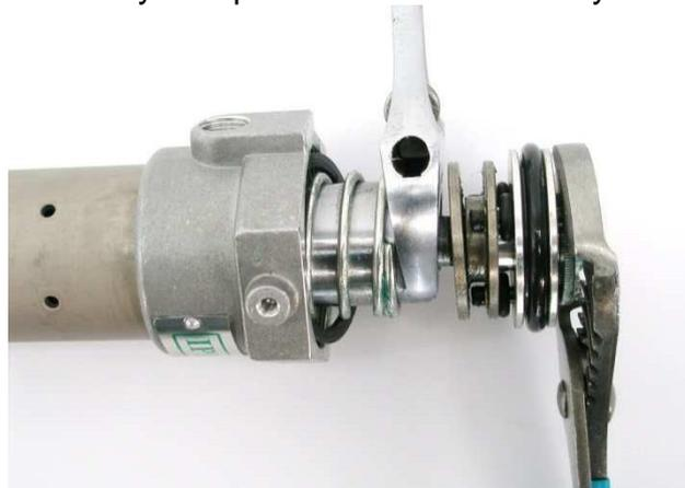
Place a pair of channel-lock pliers on the knurled area of the exhaust valve plate and a crescent wrench on the flats to remove the air piston assembly. Examine the spring in the air motor cap to ensure that it is not damaged or loose. Examine the gasket in the air motor cap and replace as needed. This gasket seals the cylinder cap to the air cylinder. Also inspect the lower return spring to ensure it is secured correctly into the air motor base assembly.
