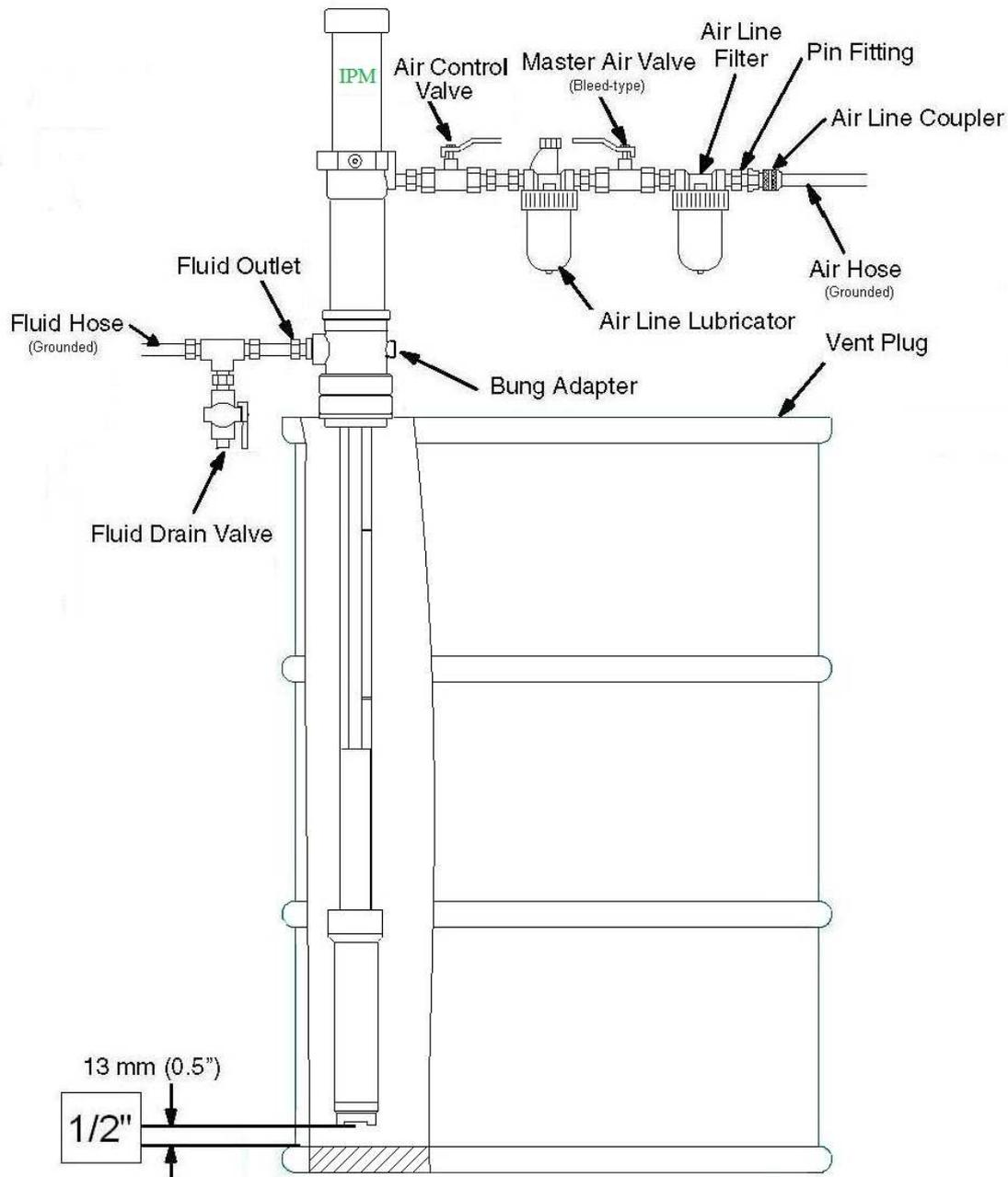
Figure B depicts only a typical installation providing a guide for your reference, but many other installation methods can be used based on your specific application. Some parts shown are not included but are sold separately. Feel free to call your **Local Distributor** for assistance.
