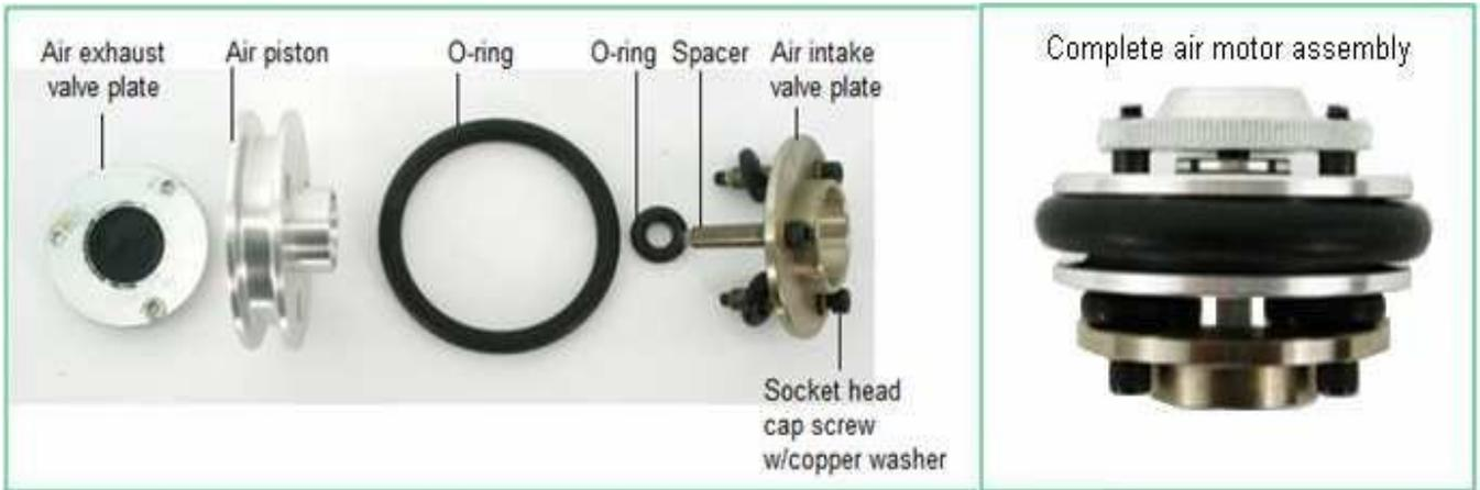
1. Assemble the air piston assembly (use thread sealant), with washer onto piston rod. Hand-tighten only.
