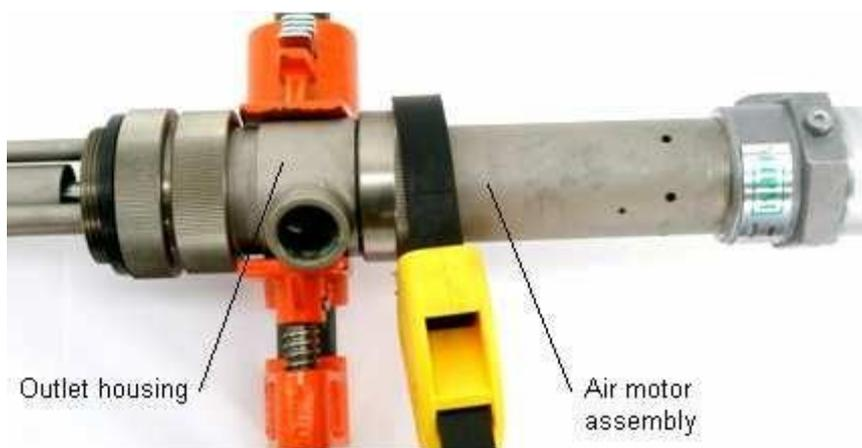
Connect the air motor section to the outlet housing as shown above.
