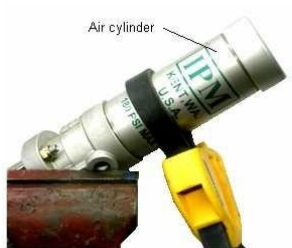
Remove the air cylinder either by hand or by using a strap wrench.
