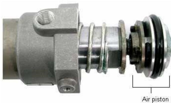
Air motor assembly and piston rod with the air cylinder removed.
