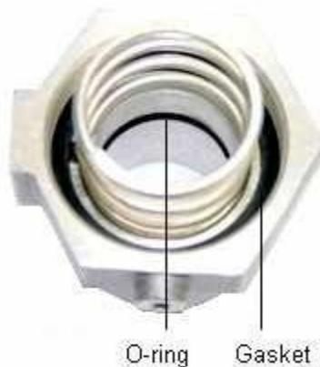
2. Place O-ring inside the machined groove in the air motor base. Place gasket in the top of the air motor base with spring centered inside the gasket, resting on the air motor base. Slide the piston rod and air valve assembly into the air motor base.
