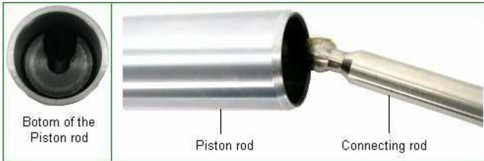
The piston rod is inside the air motor assembly- which has been removed in the above illustration so you can see more detail.
