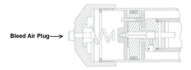
4. Place a strap wrench around the lower end of the air cylinder and carefully unthread.
