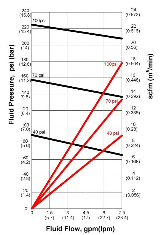
Fluid Pressure Curves (based on air input pressure 40, 70 and 100 psi)
