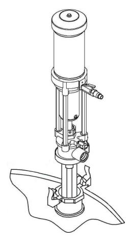
3. Attach airline onto quick disconnect fitting to complete installation. It is recommended to use a minimum 3/8" hose for the pump air supply.
