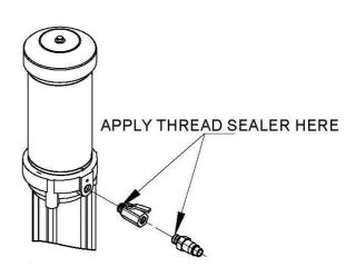
2. Screw the bung adapter onto the drum opening tightly. Carefully slide the transfer pump through the adapter and lock it in place with the bung adapter latch hooks.
