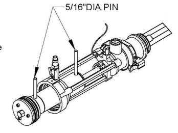
6. Remove the dowel pin from the plunger top. Air motor assembly can now be removed from the displacement plunger.
