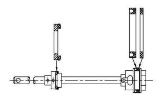
8. Inspect and replace the packings as required paying careful attention to the packing orientation.
