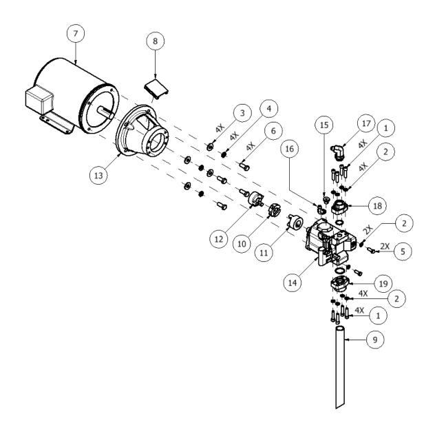
Figure 39: Motor-Line Assembly - 3 Phase
