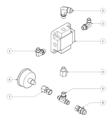
Figure 21: Hydraulic Manifold Assembly (HI-05335)
