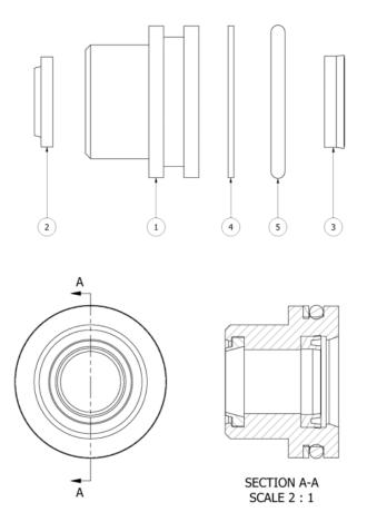
Figure 23: Hydraulic Seal Assembly
