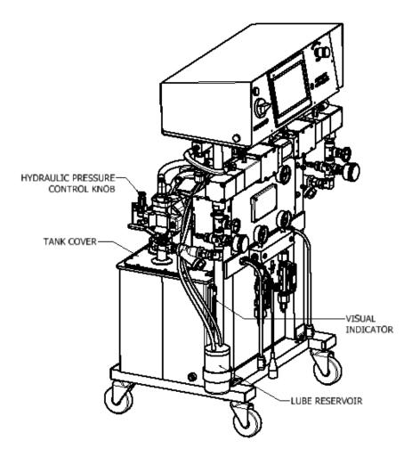
Figure 14: Component Identification - Misc
