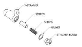
Figure 5: Y-Strainer Components
