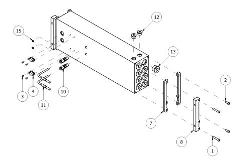
Figure 37: Heater Assembly, 8 Rod - B
