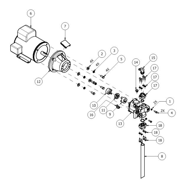
Figure 38: Motor-Line Assembly - 1 Phase
