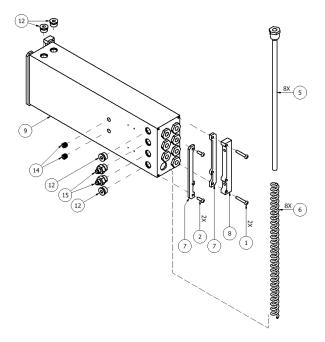
Figure 36: Heater Assembly, 8 Rod - A
