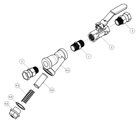
Figure 33: Y-Strainer Assembly "R" Side (YS-2)
