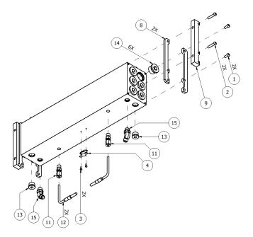
Figure 35: Heater Assembly, 6 Rod - B
