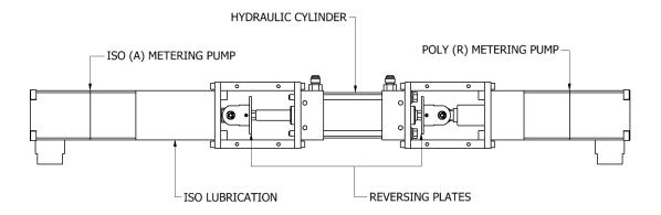
Figure 17: Metering Pump-Line (PL-9)
