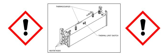
**NOTE!** The Thermal Limit Switch is a safety switch in contact with the Heater Body. If the surface temperature exceeds  $220^{\circ}F(109^{\circ}C)$  the Limit Switch will shut off the Heater power. The Limit Switch will not reset until the temperature in the Heater is below  $190^{\circ}F(88^{\circ}C)$ . The system is designed that in case of an over temperature, a contactor located in the console will open and disable power to both Heaters and the Hose.
