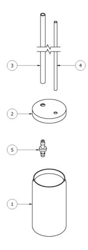
Figure 46: Lube Bottle Assembly
