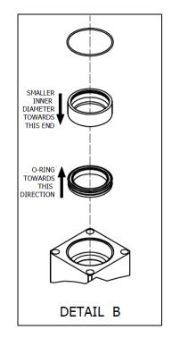
Figure 29: A & R Single Pump Assembly Detail B
