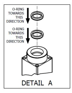
Figure 28: A & R Single Pump Assembly Detail A
