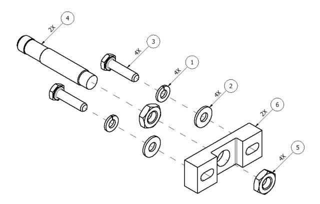
Figure 20: Prox Sensor Assembly (RM-243)
