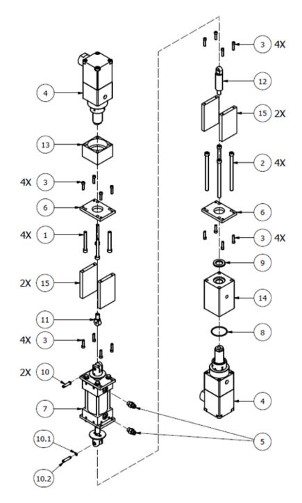
Figure 30: Pump-Line Assembly (PL-9)
