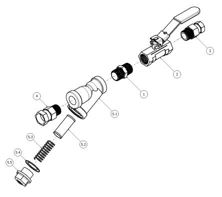
Figure 32: Y-Strainer Assembly "A" Side (YS-1)
