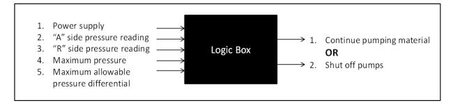
Figure 1: Pressure Balance Control Logic Diagram
