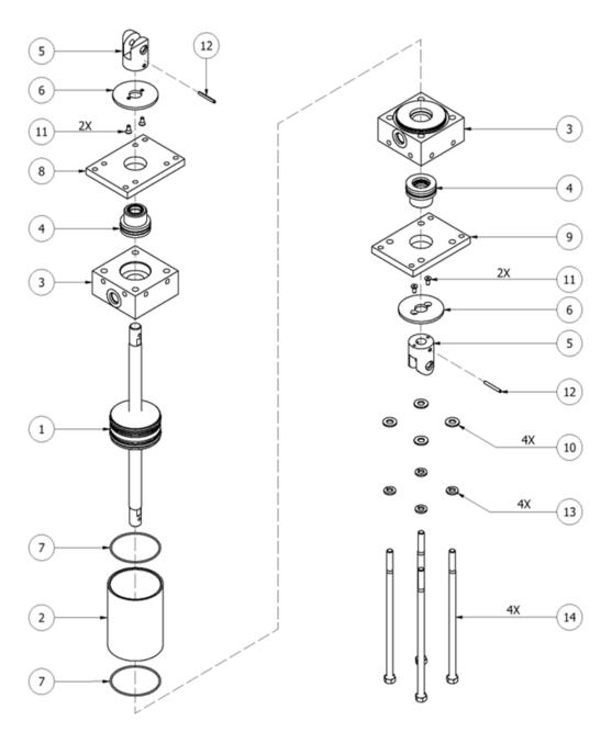
Figure 25: Hydraulic Cylinder Assembly (HI-05336)
