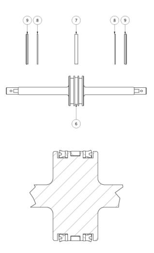
Figure 24: Hydraulic Piston Assembly
