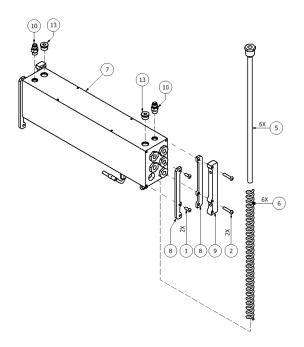
Figure 34: Heater Assembly, 6 Rod - A
