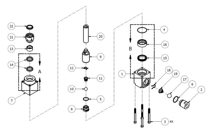
Figure 26: A & R Single Pump Assembly (202192)
