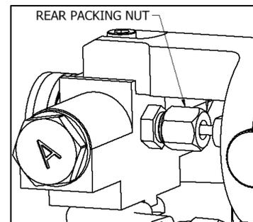
***CAUTION!*** Overtightening the rear packing nut can damage the rear packing and/or cause the Valving Rod to move slowly. *Figure 13: Rear Packing Nut*
