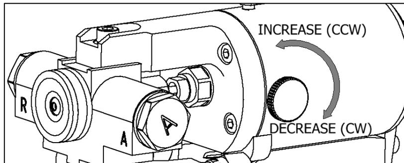
*Figure 14: Air Cap Valve Adjustment*
