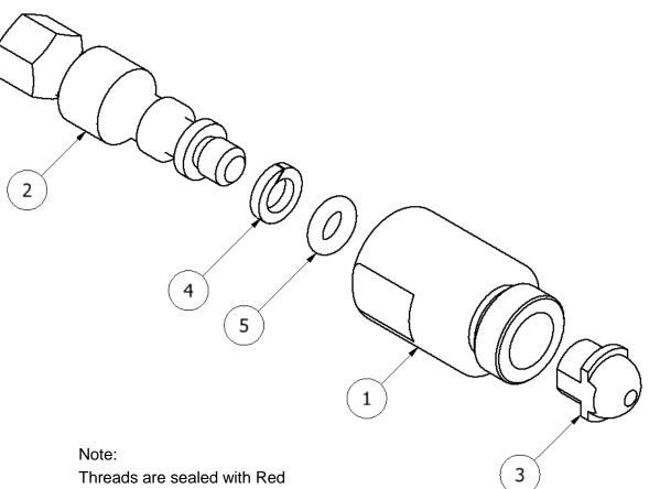
Loctite® Threadlocker and require heat to loosen
