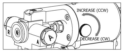
Figure 14: Air Cap Valve Adjustment
