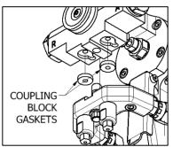
Figure 7: Coupling Block
