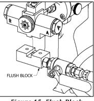
Figure 15: Flush Block Installation
