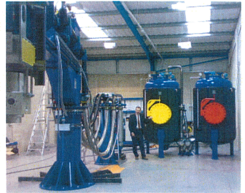
Large components tanks are required, when the moulded part weighs several hundreds kilos.
