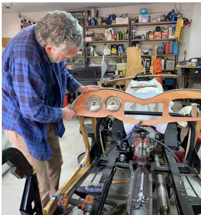
Top left, deterioration of the wood framing in the body tub; bottom left, new body timbers; top right, timber framing installed; middle right, Mike fitting a new dash made by his son of Tennessee white cherry, bottom right, primed door panels.
