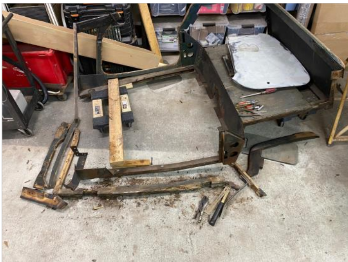
Top left, deterioration of the wood framing in the body tub; bottom left, new body timbers; top right, timber framing installed; middle right, Mike fitting a new dash made by his son of Tennessee white cherry, bottom right, primed door panels.
