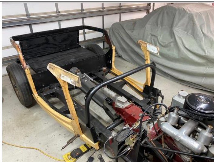
Top left, deterioration of the wood framing in the body tub; bottom left, new body timbers; top right, timber framing installed; middle right, Mike fitting a new dash made by his son of Tennessee white cherry, bottom right, primed door panels.
