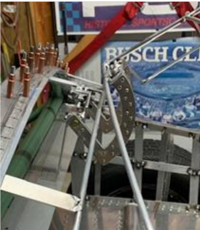
Boot lid "skeleton" and hinge assembly.
