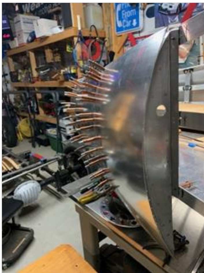
My first attempt at forming the side panels for the rear tail portion of the body.
