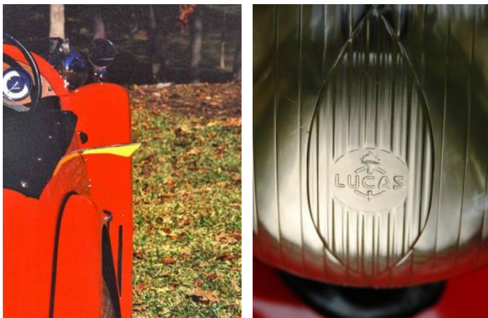
Left, the trafficator signals a right turn. Right, Lucas-crested headlamps. [All this left and right has left Ed. not in his right mind.]
