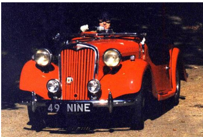
Left, the trafficator signals a right turn. Right, Lucas-crested headlamps. [All this left and right has left Ed. not in his right mind.]
