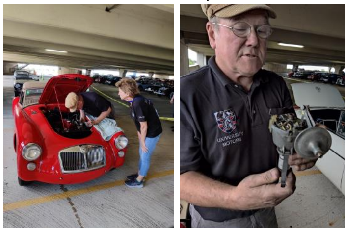
During a rolling tech session, John Twist peers under the bonnet of a bright red MGA (left) as its very interested owner looks on, and right, gets up close and personal with a Lucas D25 distributor from a 1965 MGB.
