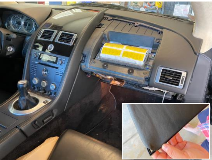
Mark's dash, with the upper panel removed and the airbag safely in place. Inset , the cut leather on the panel.
