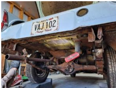
Figure 1: Gas tank out, valence removed.
