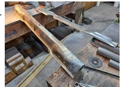
Figure 5: Rear cross member and valence prepped for installation
