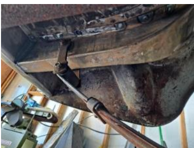
Figure 3: Driver leaf spring mount in place.
