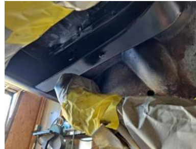
Figure 3: Driver leaf spring mount primed.
