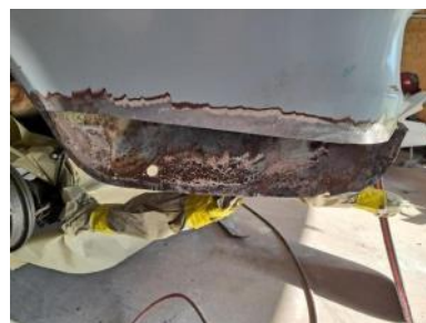
Figure 6: Rear passenger quarter panel ready for new metal.
