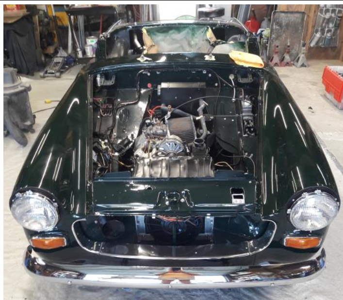
Scott Paradise often has interesting cars in his shop. About this, he says, "You don't see this every day! The long-time owner had the Wankel engine with 5-speed transmission installed some 30 years ago after hand-grenading the original powertrain. After years of fun he decided to freshen up the car. 200 hp in a Sprite . . . what could go wrong with that!?" Nothing, Scott!
