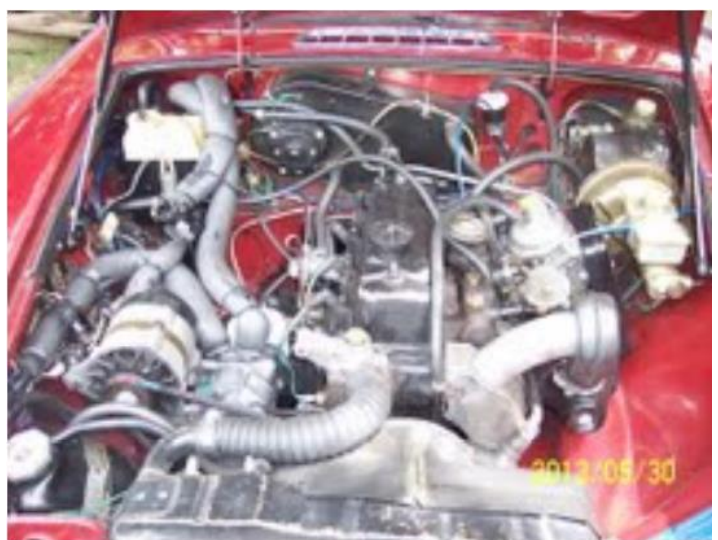
MGB with aftermarket air conditioning system.
