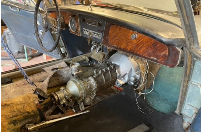
Unlike MGBs, this transmission can be removed from the cockpit.
