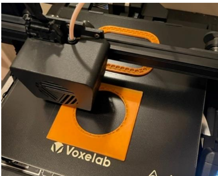
The printer in action. Note the honeycombing on the back of the part.
