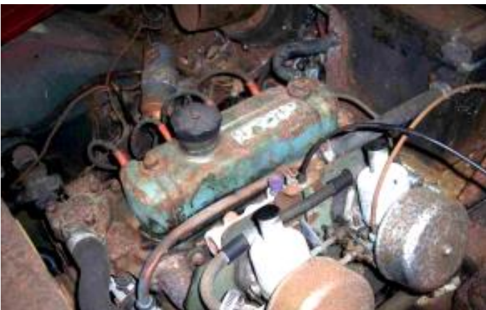
The engine of the old Sprite, showing the effects of “unplanned” storage
